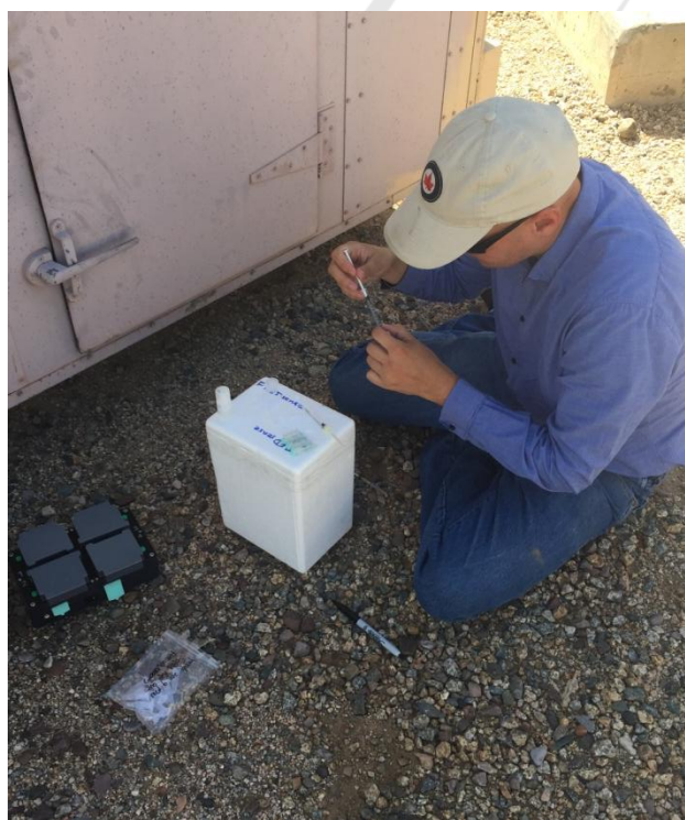
Figure 1. (Left) The FRED-Arsenic system and groundwater well sampling site, and (right) sampling of groundwater into a FRED-Arsenic cartridge before loading into the detector unit.
