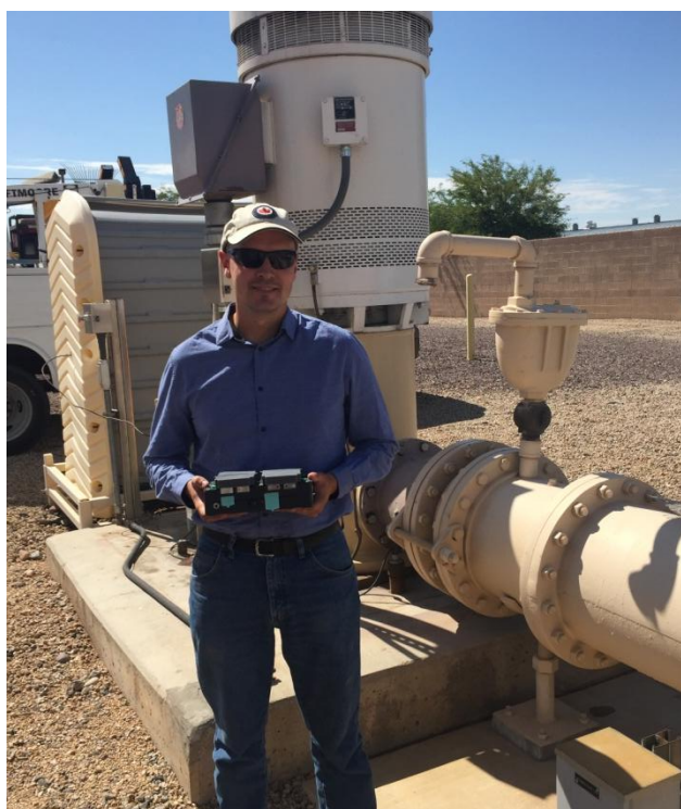
Figure 1. (Left) The FRED-Arsenic system and groundwater well sampling site, and (right) sampling of groundwater into a FRED-Arsenic cartridge before loading into the detector unit.
